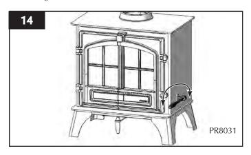
• Move the Riddling tool vigorously backwards and forwards The ash falls into the ashpan
